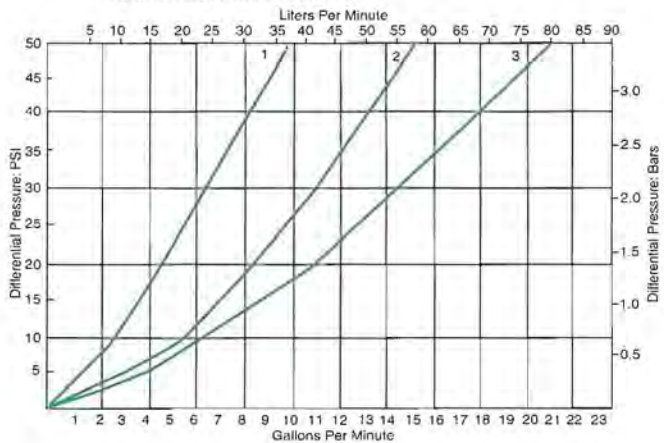
Graph 5. Pressure Drop Verses Flow: 7101 Media 100 SUS Curve 1. 331201-0000/529206-7101 Curve 2. 333201-0000/560206-7101 Curve 3. 335201-0000/562206-7101
